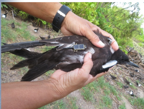
Microwave Telemetry Inc 5 g solar PTT
